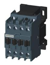
3P Power Contactor AC3:9A 1NO AC230V 50/60Hz Main circuit: Screw Auxiliary circuit: Screw
