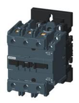
3P Power Contactor AC3:80A 1NO+1NC AC230V 50/60Hz Main circuit: Screw Auxiliary circuit: Screw
