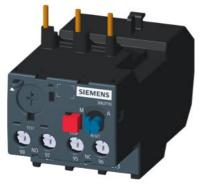
Thermal overload relay RANGE 1-1.6A Class 10 For mounting on 3MT7 contactors Size 0,1,2 Main circuit: Screw Auxiliary circuit: Screw Manual Automatic reset
