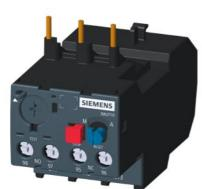
Thermal overload relay RANGE 1.25-2A Class 10 For mounting on 3MT7 contactors Size 0,1,2 Main circuit: Screw Auxiliary circuit: Screw Manual Automatic reset
