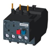
Thermal overload relay RANGE 7-10A Class 10 For mounting on 3MT7 contactors Size 0,1,2 Main circuit: Screw Auxiliary circuit: Screw Manual Automatic reset
