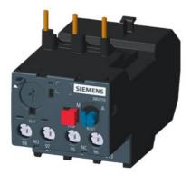
Thermal overload relay RANGE 12-18A Class 10 For mounting on 3MT7 contactors Size 0,1,2 Main circuit: Screw Auxiliary circuit: Screw Manual Automatic reset
