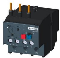
Thermal overload relay RANGE 23-32A Class 10 For mounting on 3MT7 contactors Size 2 Main circuit: Screw Auxiliary circuit: Screw Manual Automatic reset
