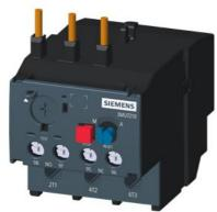
Thermal overload relay RANGE 28-36A Class 10 For mounting on 3MT7 contactors Size 2 Main circuit: Screw Auxiliary circuit: Screw Manual Automatic reset
