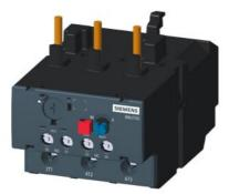
Thermal overload relay RANGE 30-40A Class 10 For mounting on 3MT7 contactors Size 3,4 Main circuit: Screw Auxiliary circuit: Screw Manual Automatic reset
