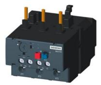
Thermal overload relay RANGE 48-65A Class 10 For mounting on 3MT7 contactors Size 3,4 Main circuit: Screw Auxiliary circuit: Screw Manual Automatic reset
