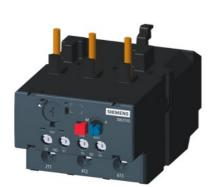
Thermal overload relay RANGE 63-80A Class 10 For mounting on 3MT7 contactors Size 3,4 Main circuit: Screw Auxiliary circuit: Screw Manual Automatic reset
