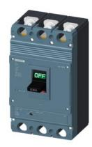
circuit breaker 3VJ1 IEC framesize 3VJ14 630A line protection ATFM 3-pole Icu=36kA@415V Ics=75% Icu In=500A overload protection Ir=400A..500A short-circuit protection Ii=10 x In Screw connection
