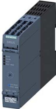
Reversing starter, 3RM1, 500 V, 0.09 - 0.75 kW, 0.4 - 2 A, 24 V DC, screw terminals
